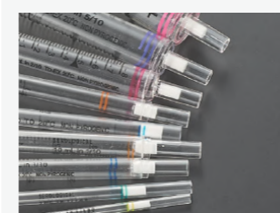
The pipet head is marked with different color codes, making the pipet range and model easy to identify
