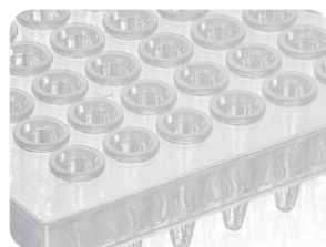
The edge of the wells is protruding to prevent cross-contamination and to facilitate sealing
