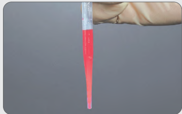
The orifice can be heat-sealed for easy carrying of liquids
